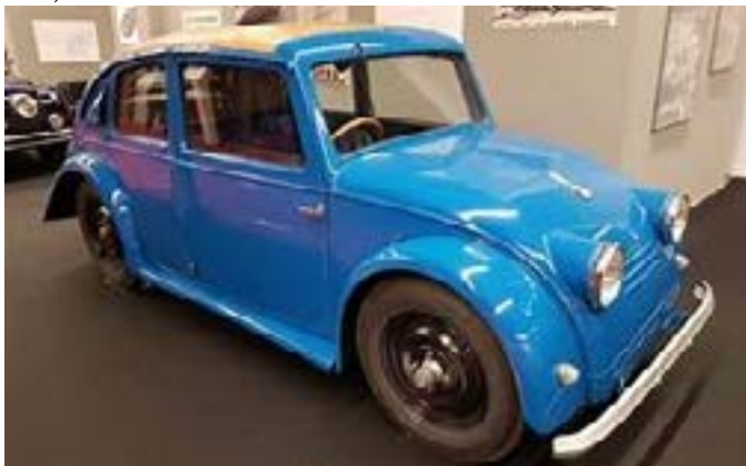
1933 Tatra V570, with air-cooled 900cc flat four
